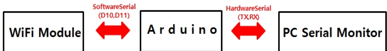
Figure 5. Experimental test for Wi-Fi wireless communication
